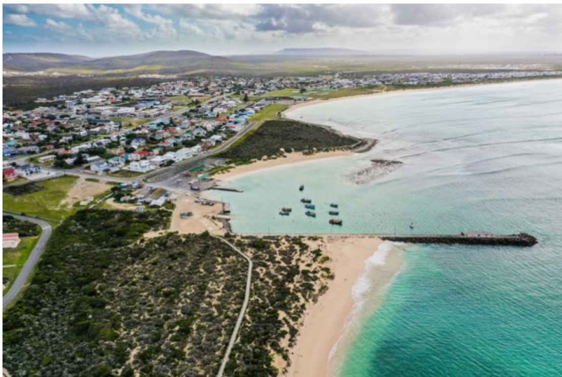
Plate 3-2: Struisbaai harbor, with sandy, well-vegetated promontories located both east and west of the harbor offering protection from swell.
